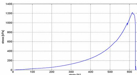
Fig. 2 Representative stress-strain curve of native HUV
