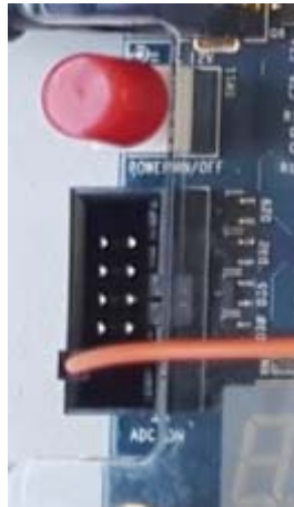
Fig. 2.1: A/D converter LTC2308 and connectors from the DE1-SoC board point of view
