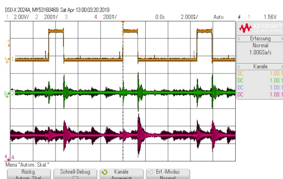
Fig. 3.1: Osci screen copies: CH1 (yellow) : pulse-width modulated input signal. CH2 (green) : voltage at 1Ω load resistor, CH3 (blue) : synchronization signal, CH4 (red) : output voltage.
