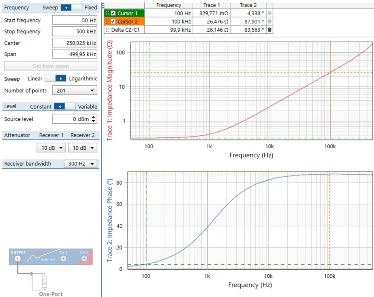
Fig. 3.2.2: Bode100 One-Port Impedance measurement of both inductors: (10+33) μH
