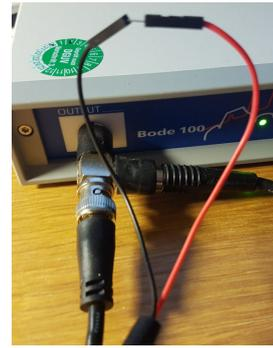
(b) Bottom: *One-Port Impedance* measurement with *Bode100*. We see a parasitic inductor at high frequencies.
