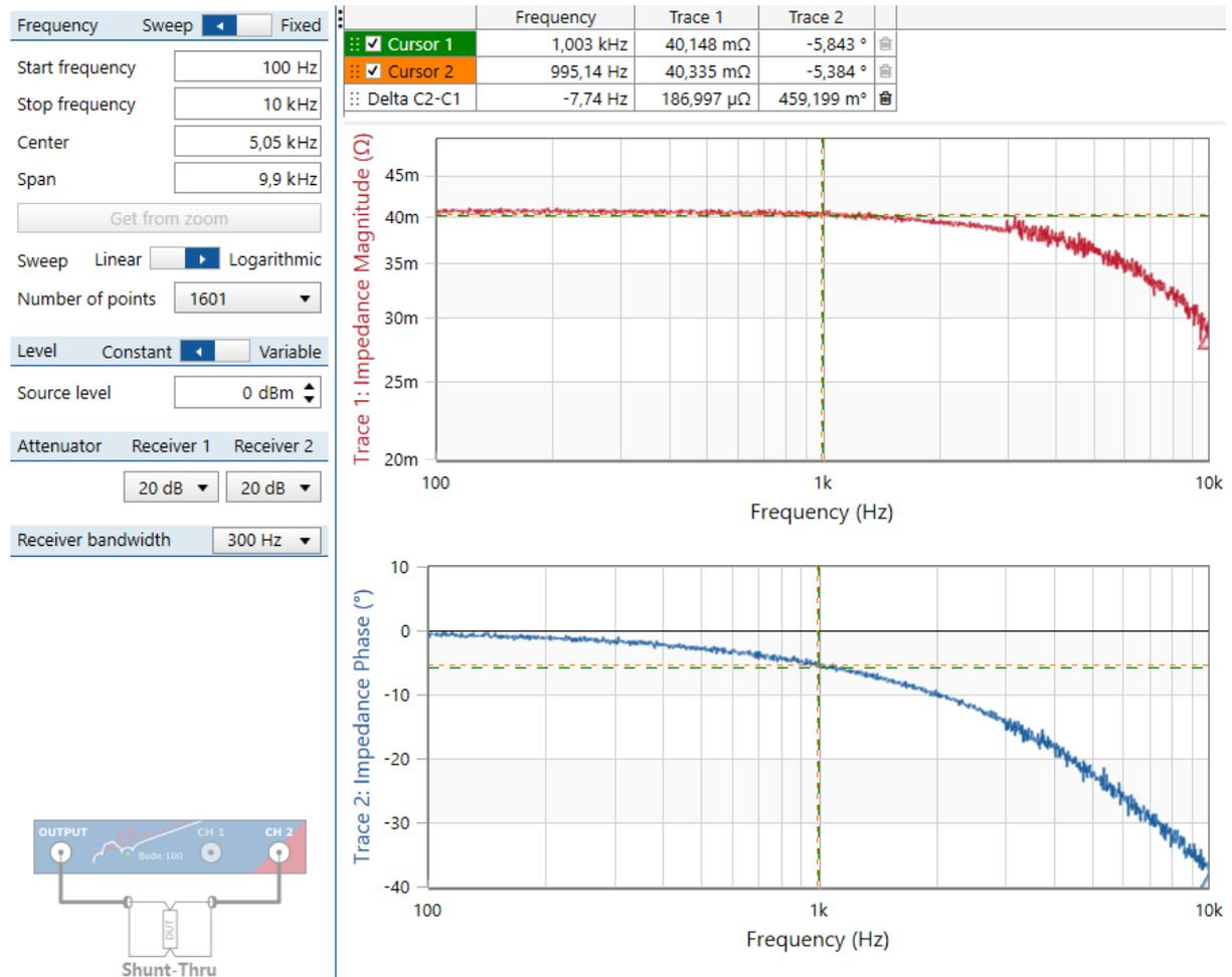
**Fig. 3.3.3(b): Bode100 Shunt-Thru impedance measurement of cables only**
