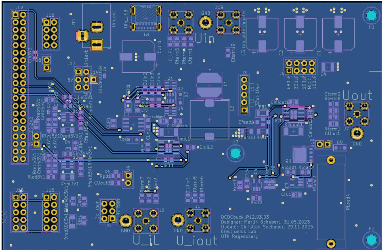
Fig. 1.4(b): DCDCbuck\_R12.03 back-side copper layer (KiCad [19])
