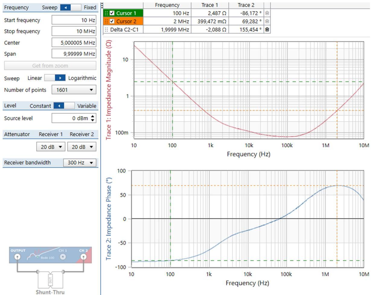
**Fig. 3.1.3:** *Bode100 Shunt-Thru Impedance* measurement of connected 680µF (nominal) capacitor connected to point *B* in Fig. 3.0.
