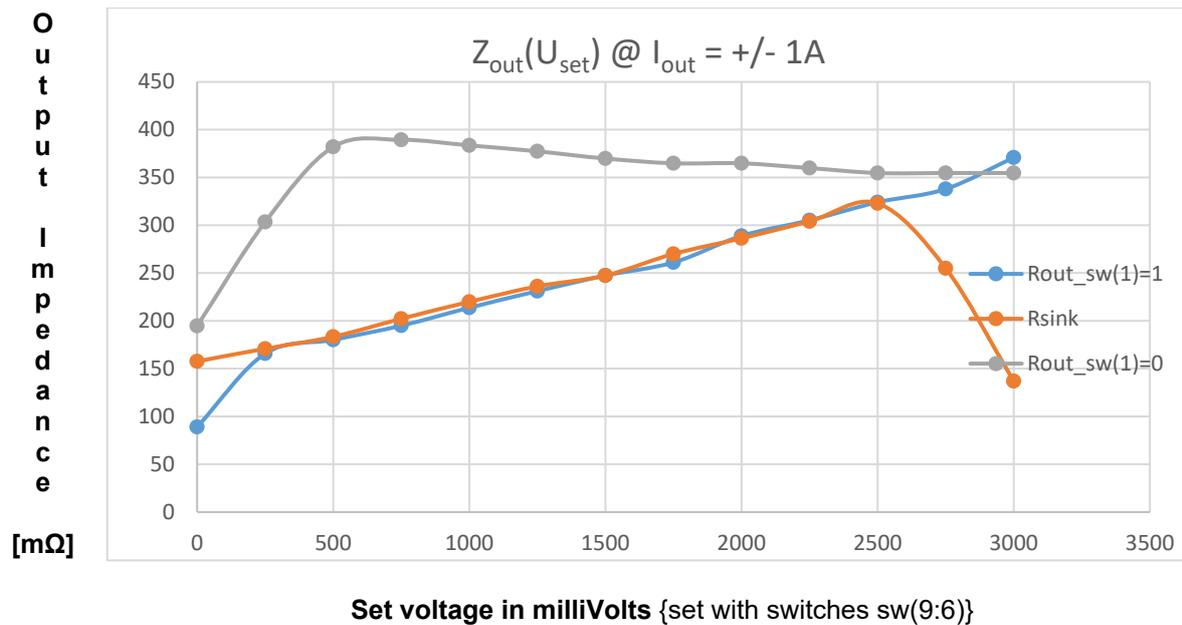
**Fig. 4.2.2:** DC output impedances measured for a *DCDCbuck* circuit in 3 different modes of operation: blue: synchronous current source, yellow: synchronous current sink/drain, grey: asynchronous current source. Measured was the voltage drop from  $I_{out}=0$  to  $\pm 1A$ .
