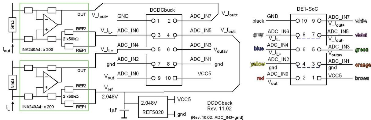
**Fig. 1.5:** Pin assignment of the 10-pin ADC input plug (connected by the 10 wire ribbon cable). It is a cross cable! Color code valid for  $V_{CC}(ADC) = \text{black}$ . Numbers within the plug-box are the pin-numbers of the plug. Labels  $ADC\_IN\#$  ( $\# = 1 \dots 8$ ) indicate input channel number  $\#$  of ADC *LTC2308* [15].  $ADC\_IN3$  is ground for board revisions  $Rev \leq 11.01$ .
