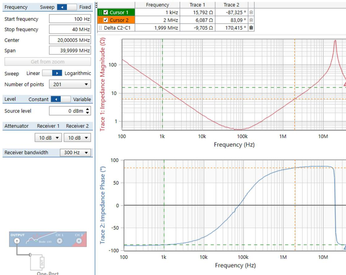
**Fig. 2.8.3:** *Bode100 One-Port Impedance* measurement of a capacitor of nominal 10 μF.
