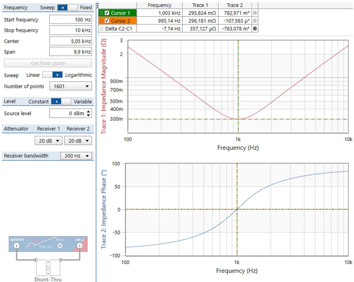
**Fig. 3.3.3(a):** Bode100 Shunt-Thru impedance measurement: point A in Fig. 3.0 versus ground.
