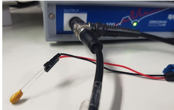
(b) Bottom: *One-Port Impedance* measurement with *Bode100*. We see a capacitor at low frequencies and a parasitic inductor at high frequencies.
