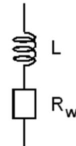
**Fig. 2.1.2:**  $L, R$  in series which models a real-world inductor.
