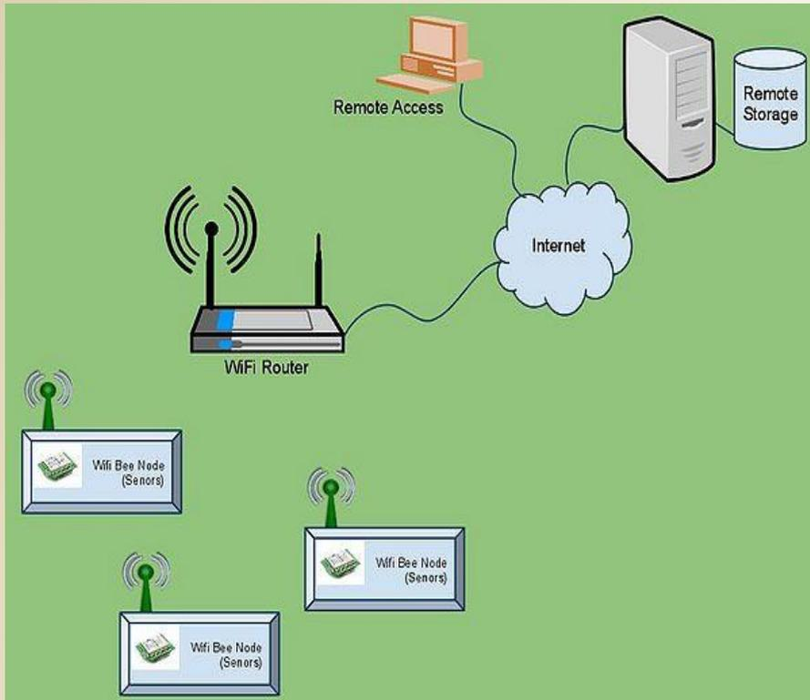
The architecture of Solar Powered Wireless Sensor Network.
