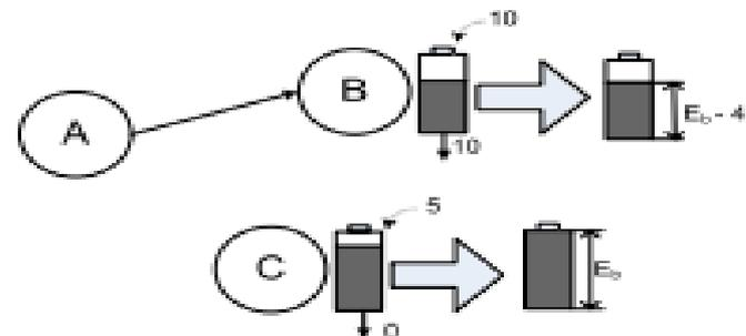
(c) Battery status of node B and C after B relayed 5 packets within 5 seconds
