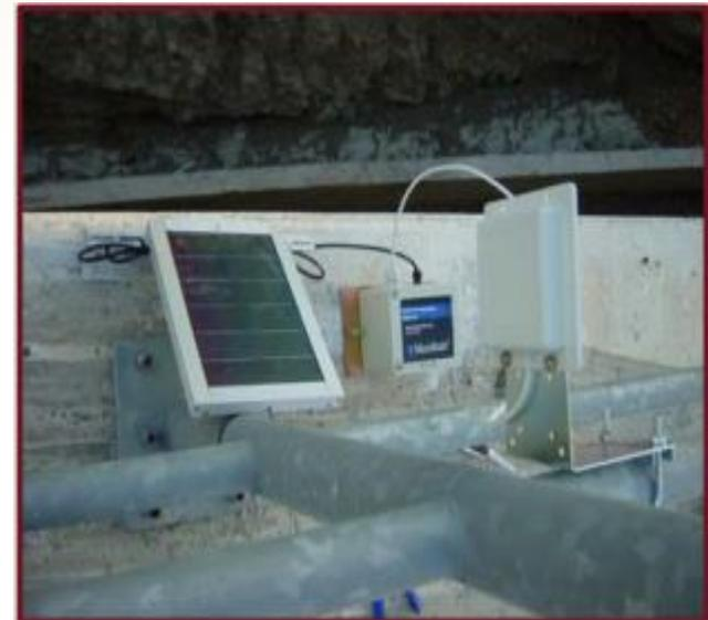
Solar Energy Harvester for Civil Structural Monitoring
