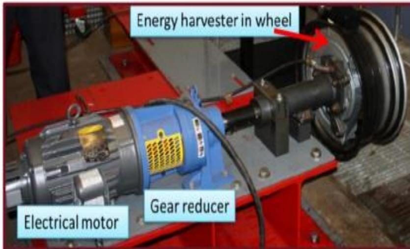
Rotating Energy Harvester for Tire Pressure Monitoring
