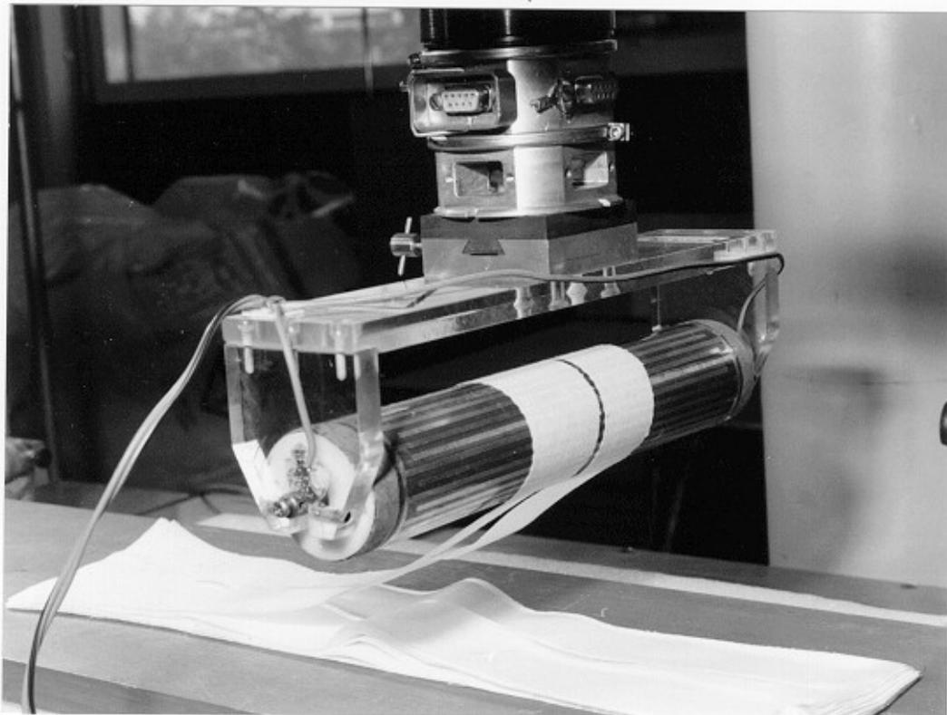
This allows the uppermost panel to be peeled from a stack leaving the others undisturbed and ready for the next prehension cycle<sup>16</sup>.
