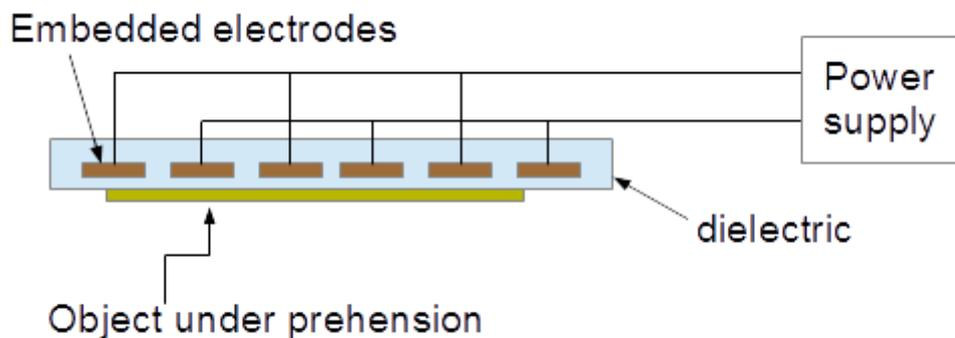
The principle of electroadhesion can be basically split into 2 different principles: When used to prehend electrically conducting objects the basic Gauss theorem may be used:
