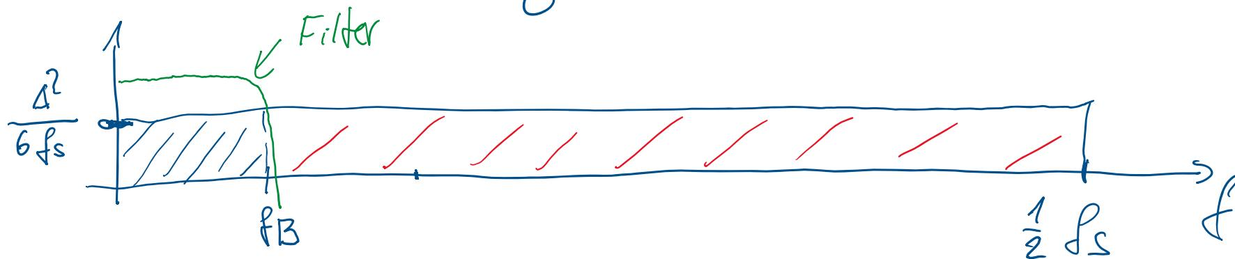
Quantization noise in Base band  $0 \dots f_B$
