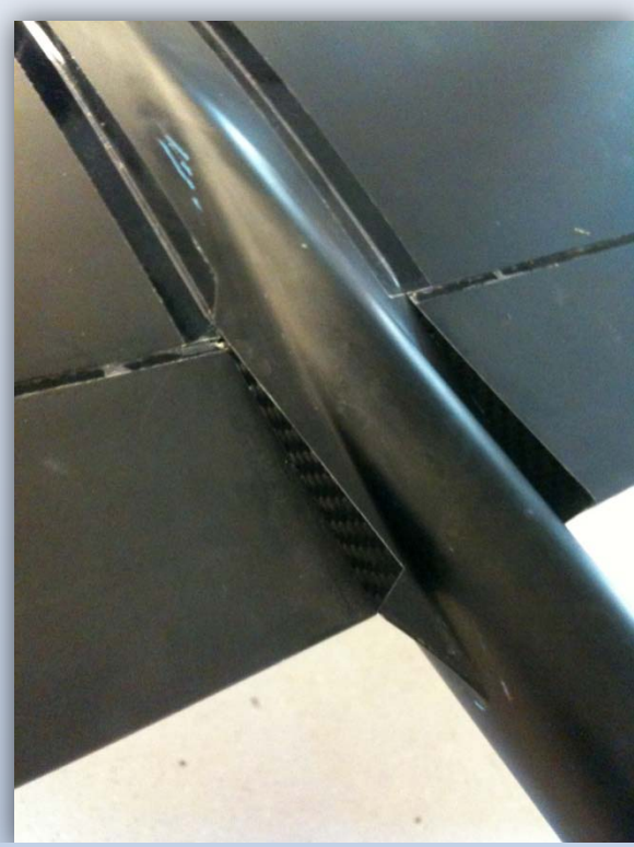
Fig. 3: drag reduction with guiding plates
