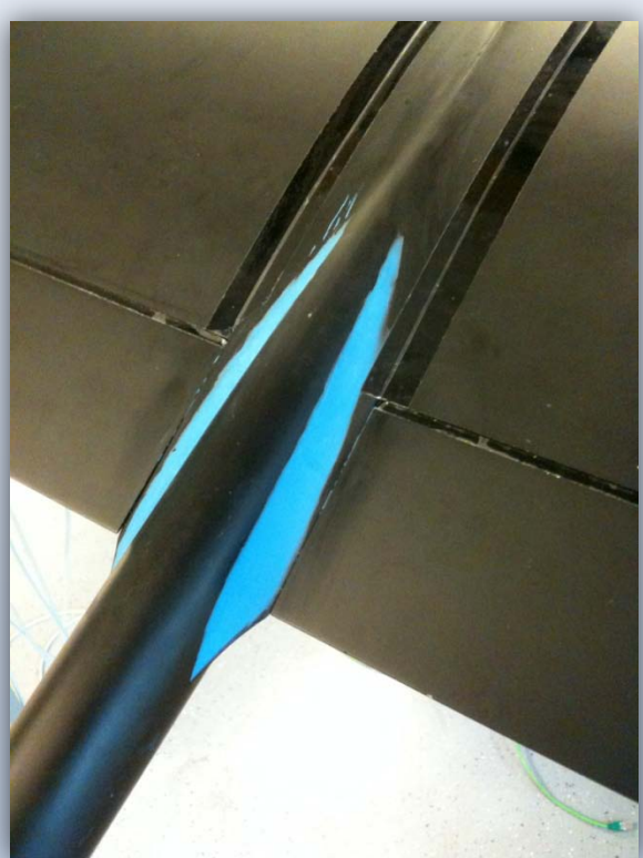
Fig. 1: drag reduction with corner arc
