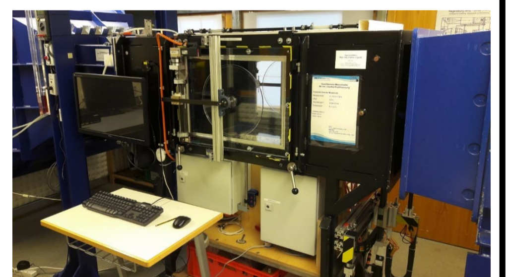
Fig. 7: Polamax closed wall test section of the RWT
