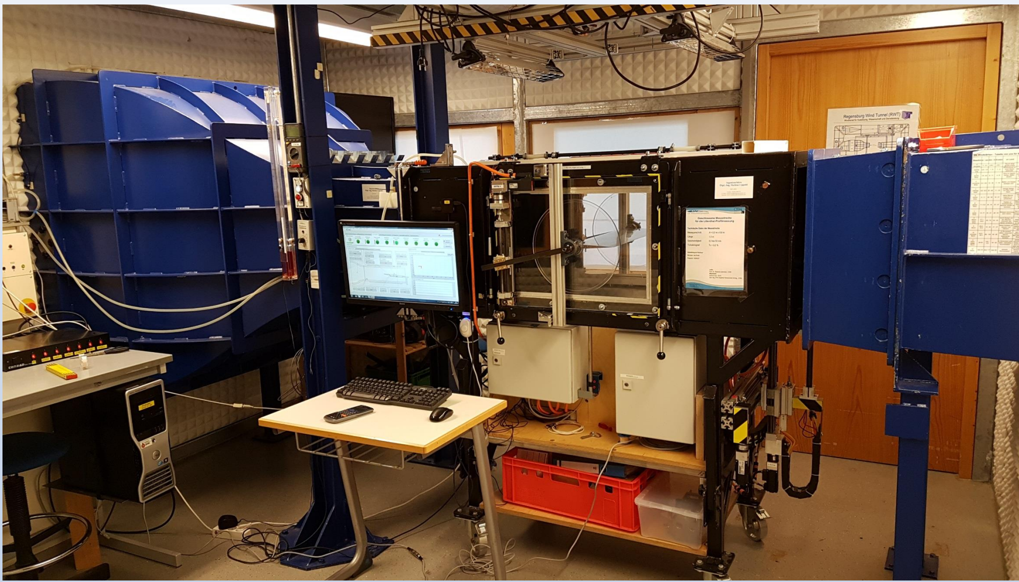
Fig. 1: Closed test section in the Regensburg Wind Tunnel (RWT) at the OTH Regensburg.
