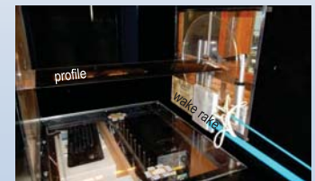
Fig. 4: The RG-15 airfoil in the closed test section of the RWT
