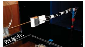
Fig. 3: Turbulence measurement setup in the closed test section
