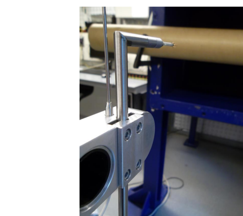
Fig. 5: Dantec reference measurement system placed in the wake of a cylinder (Probe P55R62)
