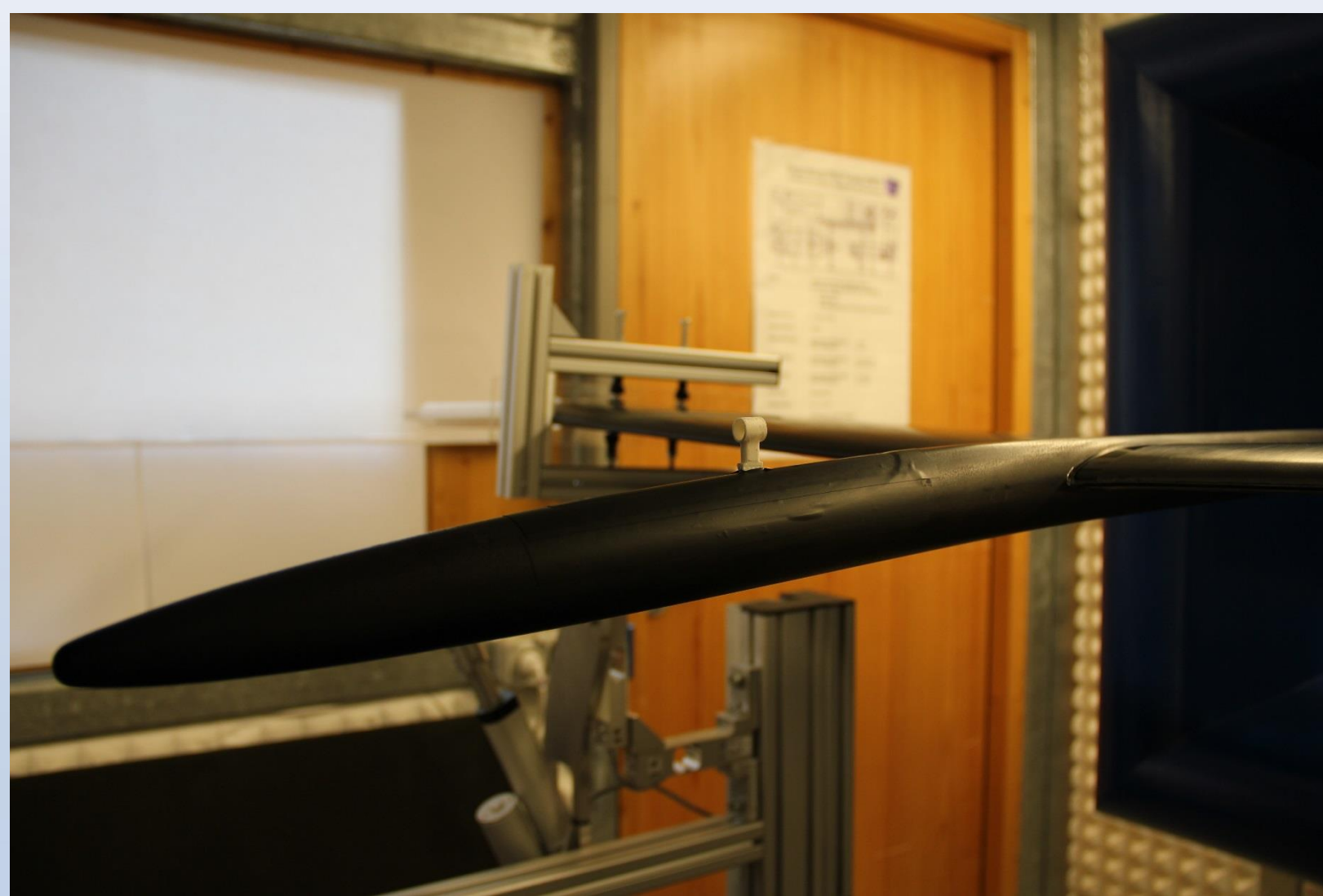
Fig. 1: The mounted differential pressure probe on top of the aircraft.
