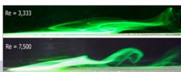
Fig 8. Sideview at Re = 3,333 (top) and Re = 7,500 (bottom) with H = D and S = 2.5 D .
