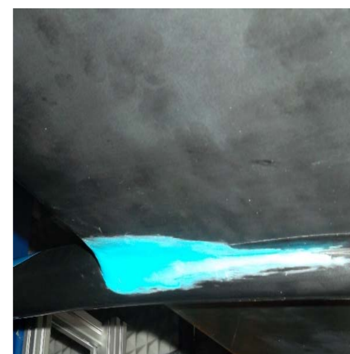
Fig. 6: shaping FG_S1 applied on the model
