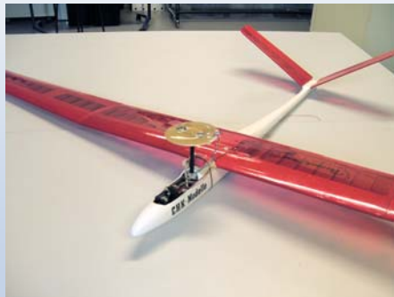
Glider with SondenUFO, GPS, temperature probe and data logger
