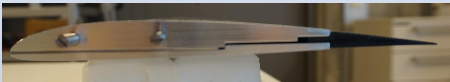
Fig. 1: Side view of the metal MM17-240 0.5mm airfoil. The trailing edge (in black) is made out of plastic and has been 3D printed, whereas the other parts have been milled.
