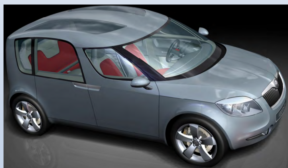
Fig. 2: Design study Skoda Roomster using a tangential A-pillar transition
