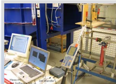
Fig. 2: Measurement equipment for detecting the boundary layer with a microphone
