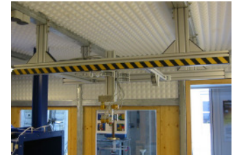
Fig. 5: the 6-component-balance in the measuring cabin of the RWT
