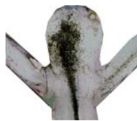
Visualisation of flow using the hydrogen bubble method
