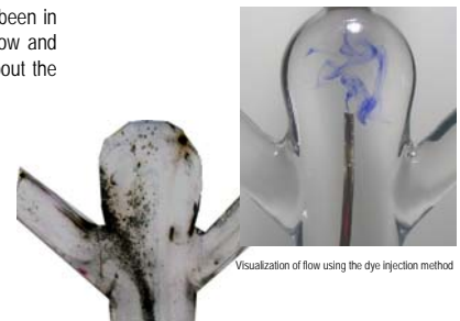
Visualisation of flow using the hydrogen bubble method
